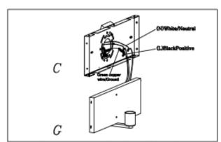
Step.2:Wire fixture to wires in outlet box.Freen copper wire is for ground.And carefully position all wires inside the outlet box.
