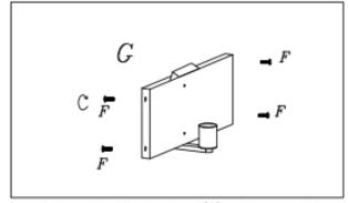
Step.3:Place the fixture body(G)against mounting bracket, Align the two holes of the mounting bracket and fixture body, then tighten the screws(f).
