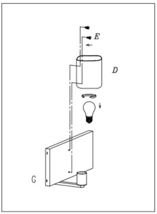
Strp.4:Align the glass with the holes in the backplate and secure with ball nuts provided.
