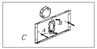
Step.1:Fasten the mounting bracket(C)onto the outlet box using two outlet box screws.
